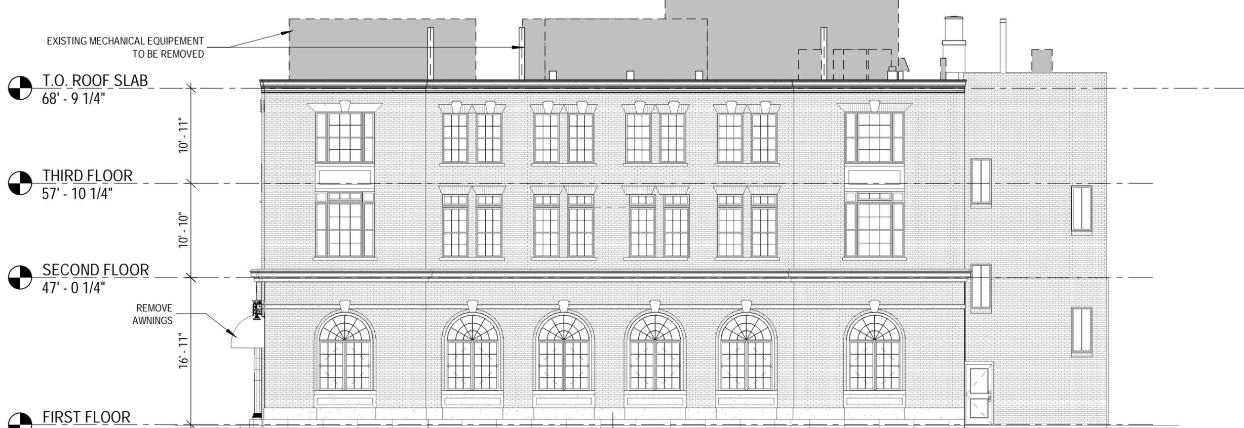
1 SOUTH ELEVATION - EXISTING
