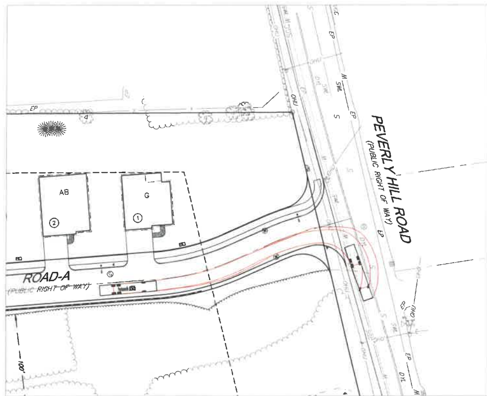
FIRE TUCK TURNING FROM ROAD-A SOUTHEAST ONTO PEVERLY HILL ROAD
