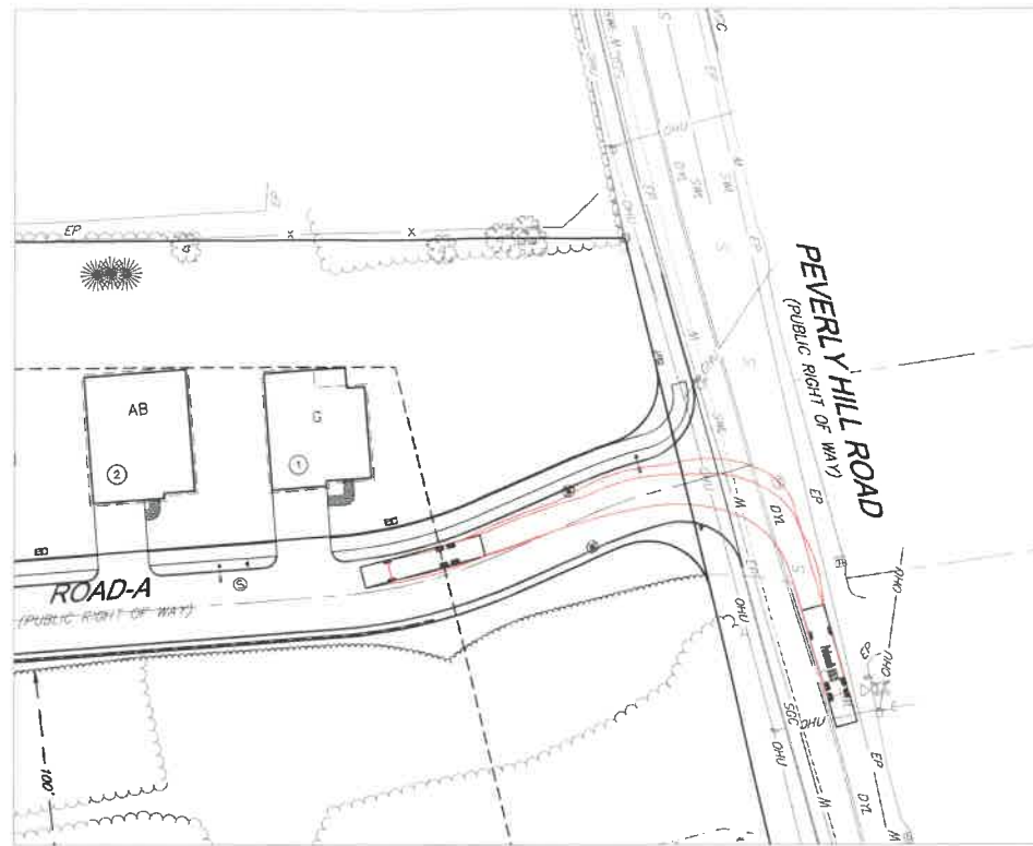
FIRE TUCK TURNING FROM PEVERLY HILL ROAD NORTHWEST ONTO ROAD-A
