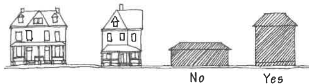
The one-story residence is not appropriately scaled nor does it have appropriate form and massing for the streetscape. The form has a horizontal rather than vertical emphasis. The building to the right has a similar scale and form to the existing buildings.
