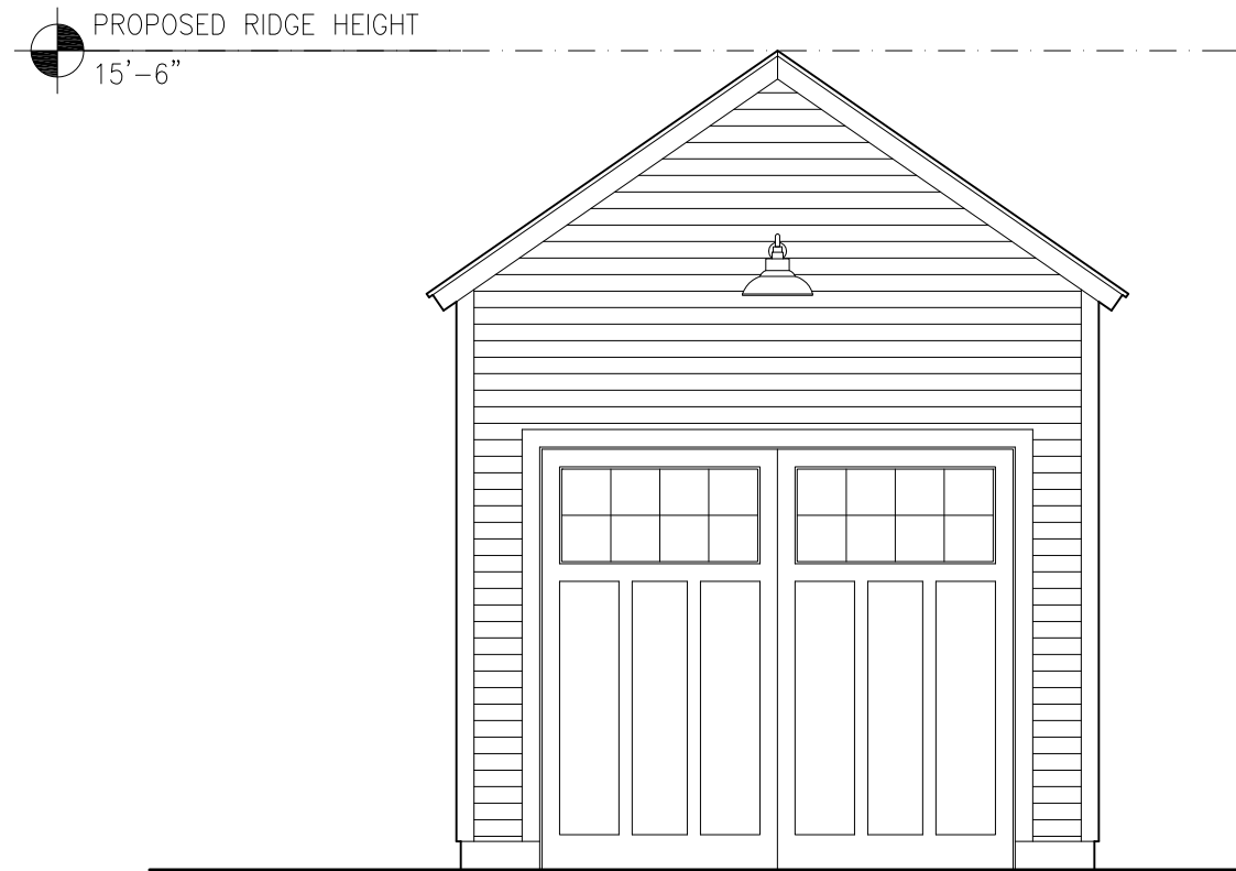
PROPOSED NORTH ELEVATION SCALE 1/4" = 1'-0"
