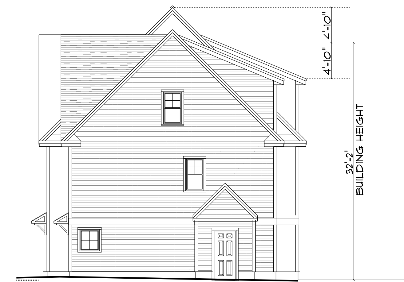
TYPICAL SIDE ELEVATION BUILDING B TYPICAL FOR UNITS 1-3 AND 4-6 (WITH SPRINKLER ROOM)
