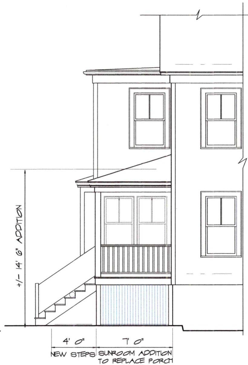
LEFT SIDE ELEVATION AT SUNROOM SCALE: 3/16" = 1'-0"
