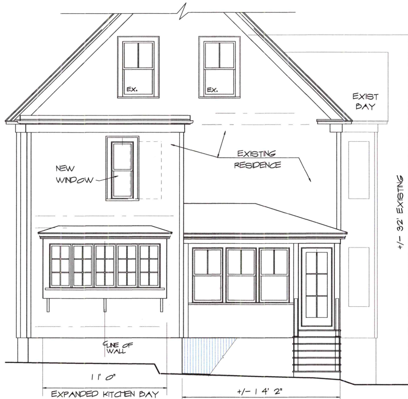
REAR ELEVATION SCALE: 3/16" = 1'-0"
