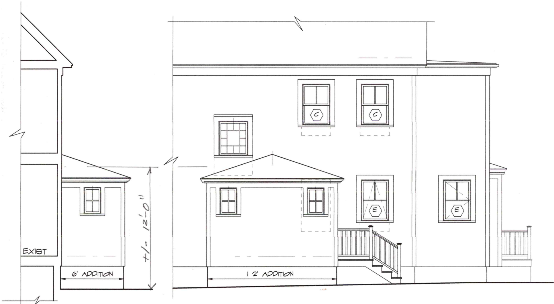
MUDROOM ADDITION FRONT & RIGHT SIDE ELEVATION AT DRIVEWAY SCALE: 3/16" = 1'-0"
