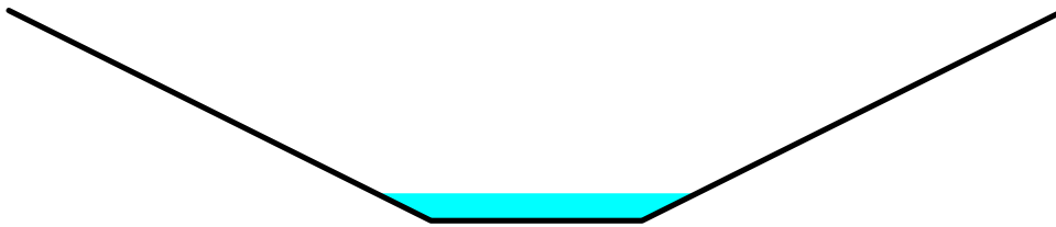
Reach 5R: Grass Swale
