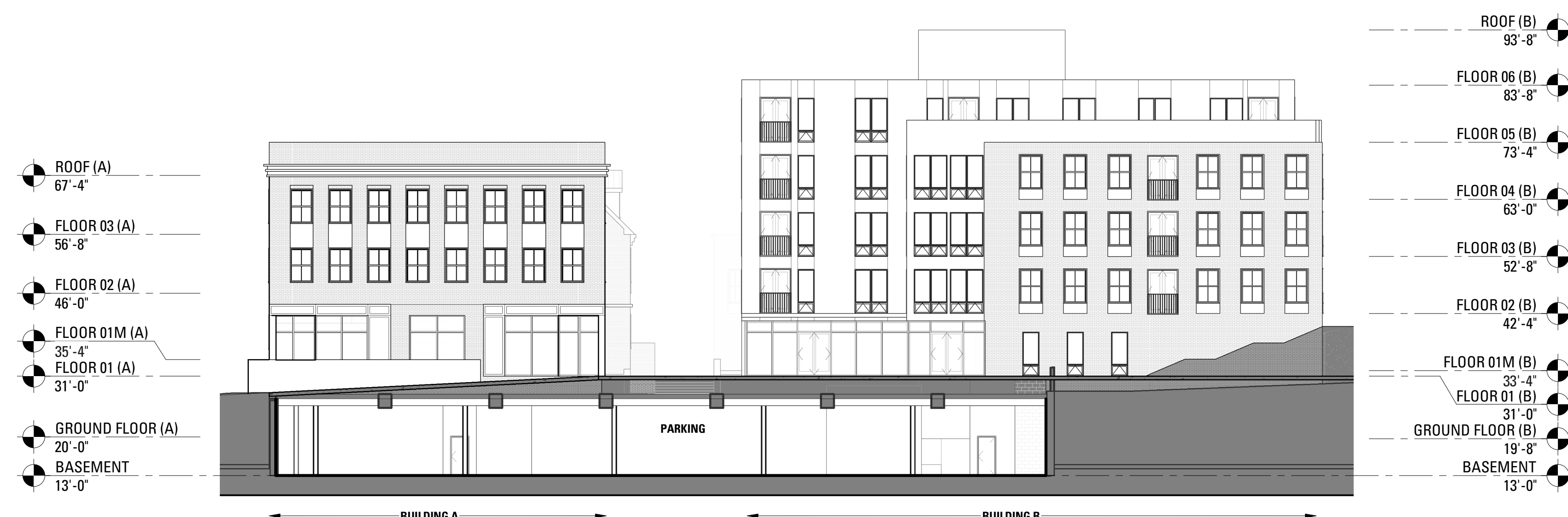
2 SOUTH (LINDEN WAY) ELEVATION SCALE: 1/16" = 1'-0"
