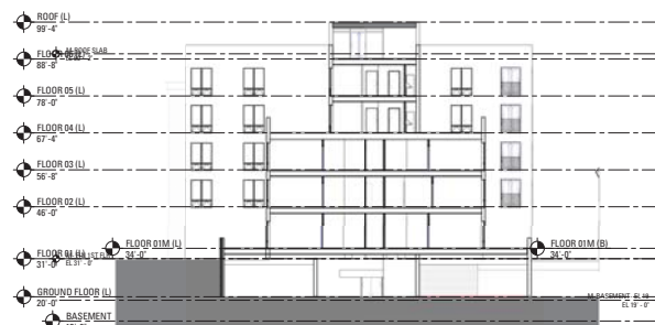
4 "LINDEN WAY" RESIDENCE - NORTH ELEVATION (INTERIOR) SCALE: 1/8" = 1'-0"
