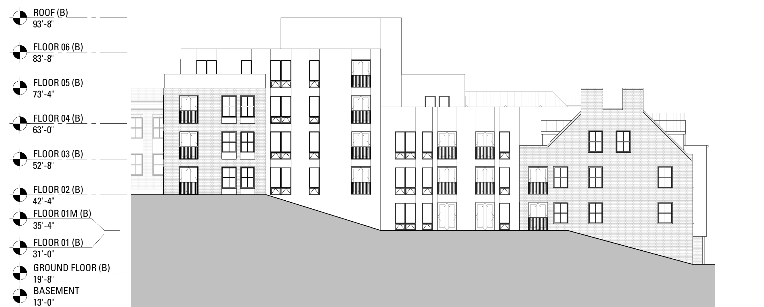
4 BUILDING B - EAST ELEVATION SCALE: 1/16" = 1'-0"
