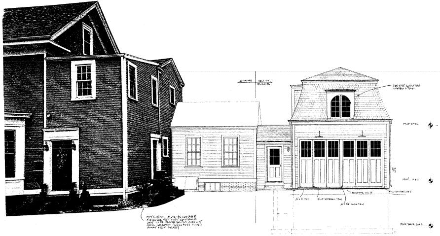
PROPOSED WEST ELEVATION, LEFT SIDE FROM IS UNGTON ST. SHOWING HEW, B'WINDOW.
