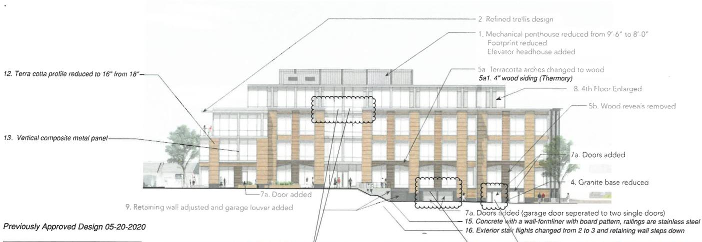
A. Aluminum metal panel instead of glass at 4th floor window bay. The roof coping returns to the wall and cannot terminate against glass. This was a constructability issue.
