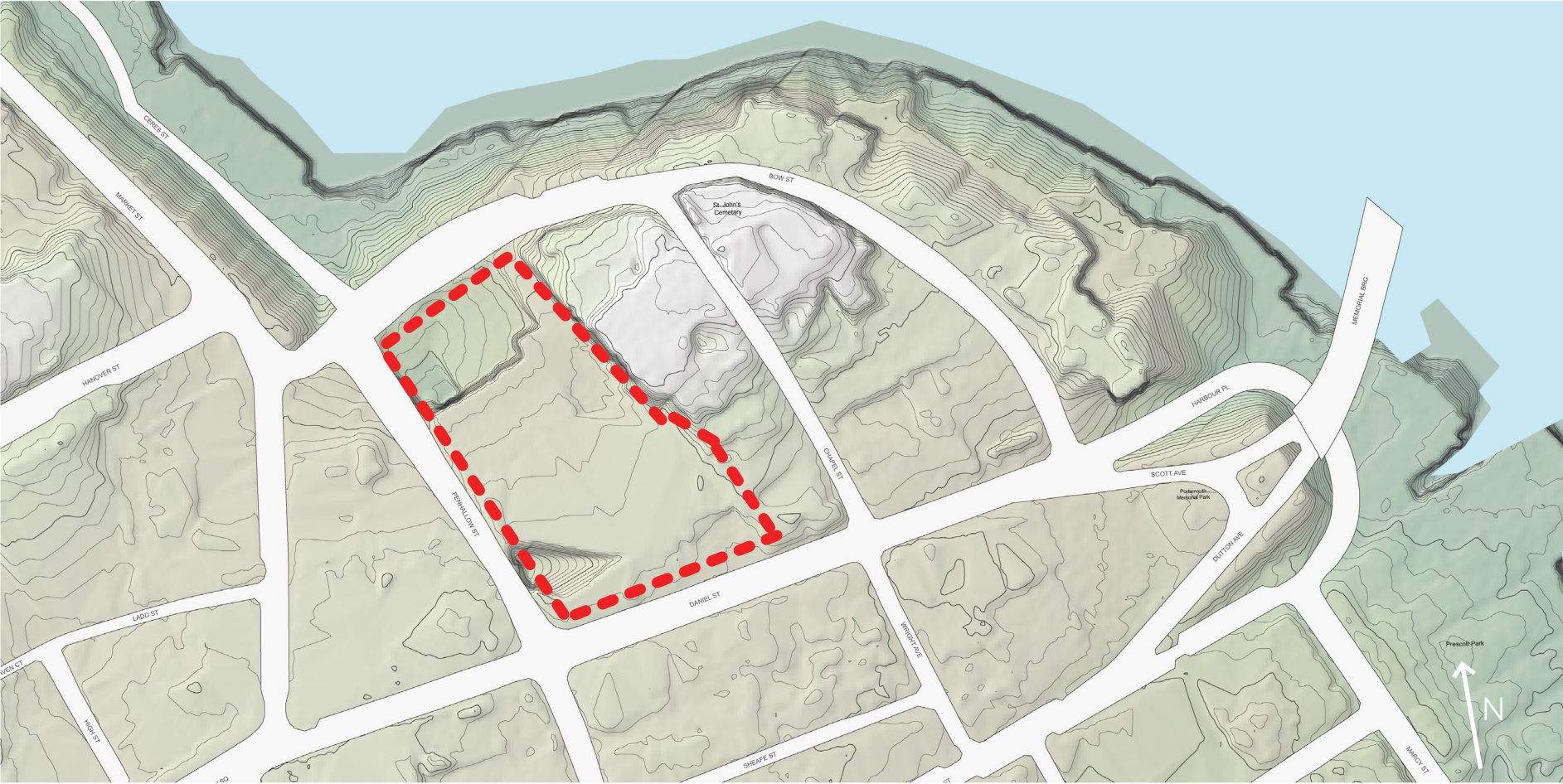
The McIntyre site features a significant grade change between Daniel Street (FF= 31 feet elevation above sea level) where the Main Building and One-Story Section are located and Bow Street (18 feet elevation), which is approximately equal to one-story of a standard office building. St. John's Church is approximately 46 feet elevation above sea level.
