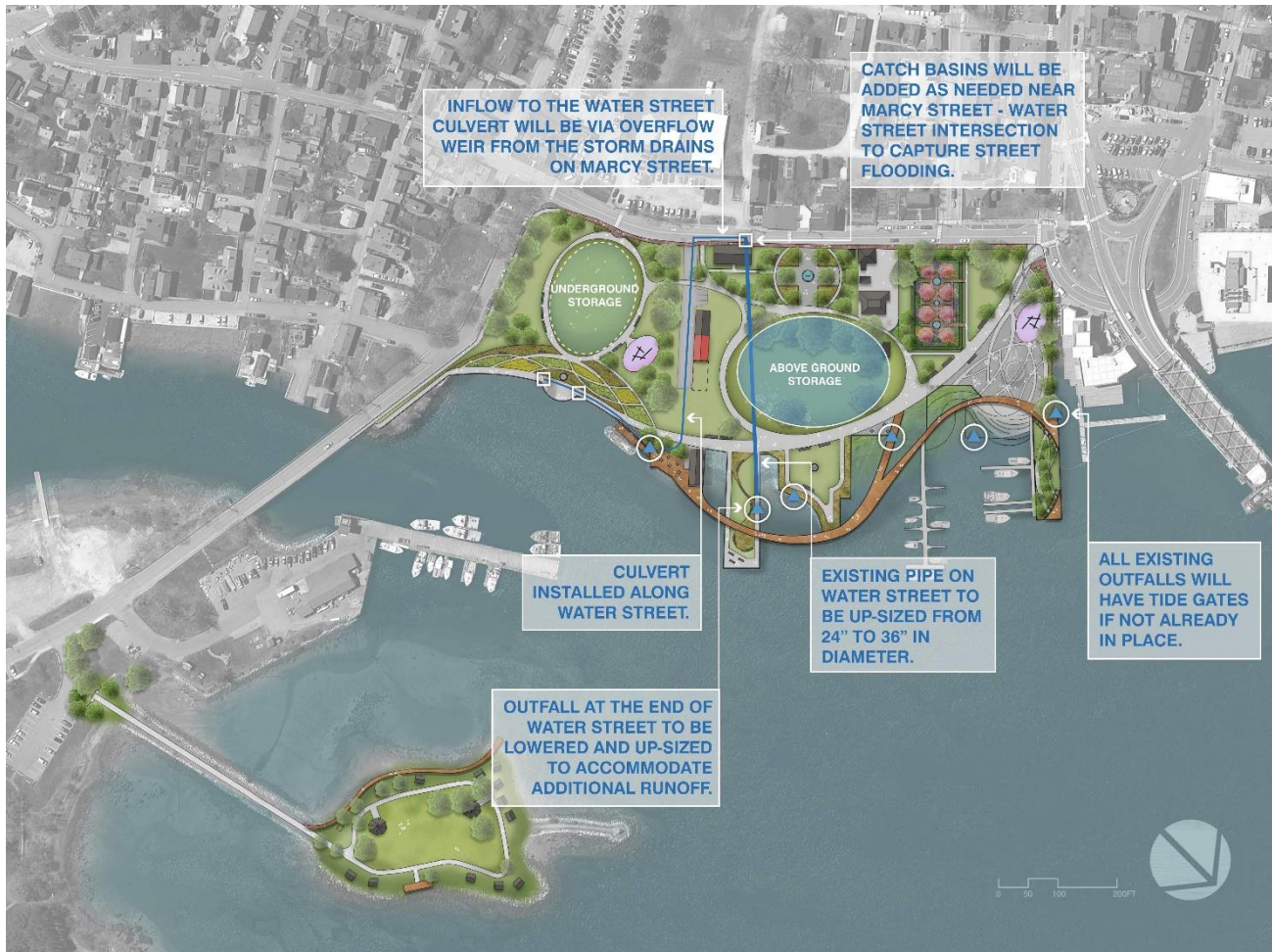
Figure 2. Proposed stormwater infrastructure improvements at Prescott Park
