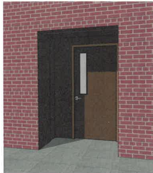
New recessed single panel door with vision window for employee safety and ADA accessible hardware. Paint to match existing on 2'-6" recessed walls and door exterior.
