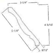
5-1/4" CROWN #5045K Projection: 3-1/4" Height: 4-3/16" Spring Angle: 37° 9/16" x 5-1/4" x 16'
