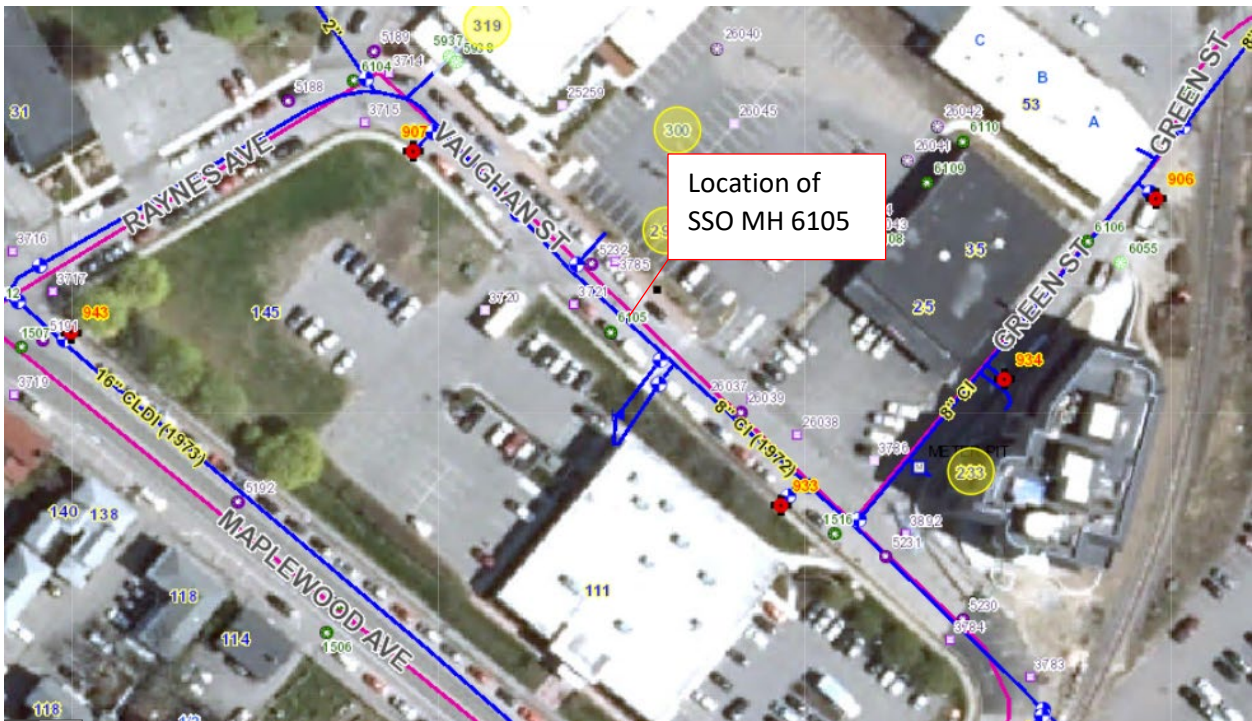
Site Map: Manhole 6105 and the flow discharged into catch basin leading to North Mill Pond
